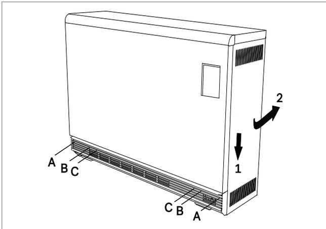
7.3 Remove the screws (A) for the side panels. Push the side panels down (1) and swivel them out (2). After removing the side panels, loosen the fixing screws (B) for the front panel. Do not loosen the screws C.
