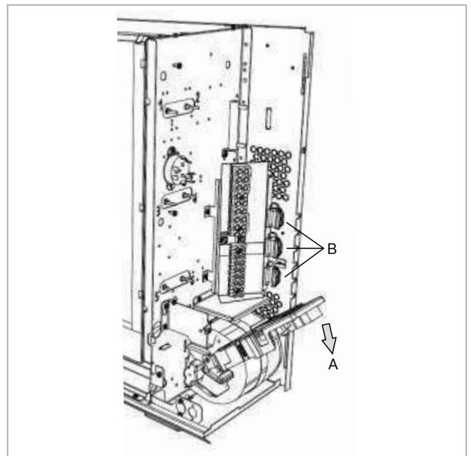
8.1 Fold the main electronics down by 90° (A) to access the connecting terminals.
