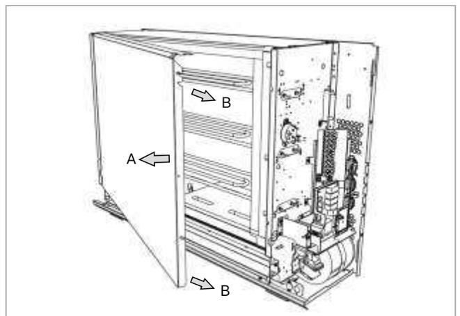
7.6 Remove the core room cover. To do this, loosen the three fixing screws at the side. Lift the core room cover slightly, swivel it outwards (A) and then pull it to the right (B).
