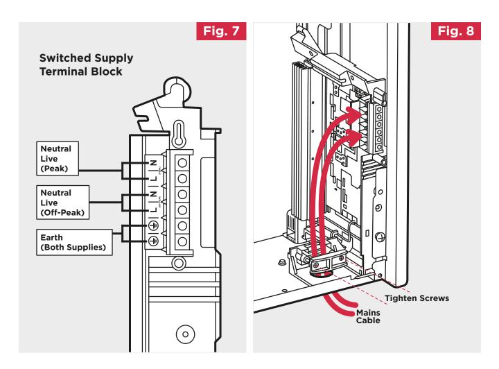
**8.** The mains cable entry and terminal block will be visible on the right hand side of the unit. Insert the mains cables through the cable gland at the bottom of the heater in readiness for connection (**Fig. 8**).
