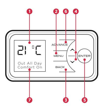
The heater is fitted with an adjustable thermostat enabling the room temperature to be controlled. The **minimum** room temperature is 7°C. The **maximum** temperature is set to 26°C. A temperature of 21°C represents a **normal** room temperature.
