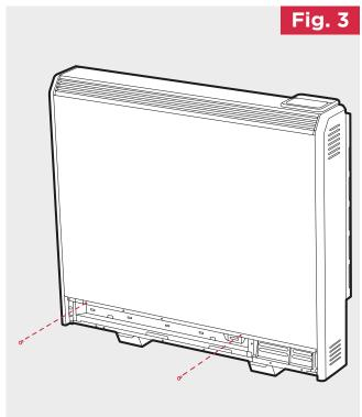
Ensure the back of the heater is flush against the wall. If the skirting board is taller than 120mm and deeper than 15mm it should be cut to accommodate safe installation of the heater.
