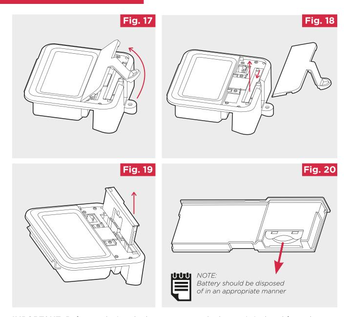
**IMPORTANT:** Before replacing the battery ensure the heater is isolated from the electricity supply.
